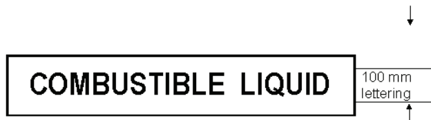
Figure 5—Placard for C1 combustible liquids
